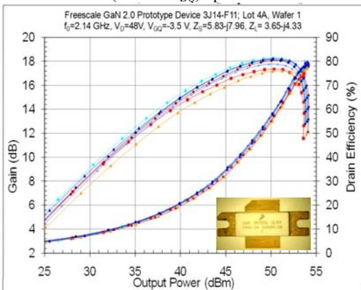
Figure 9: Saturation characteristics over power for a single 37.8 mm die in a NI-780-2 package under 2.14 GHz, 48V pulsed RF class C operation. Device is biased at -3.5 V (0.5 V below threshold).
