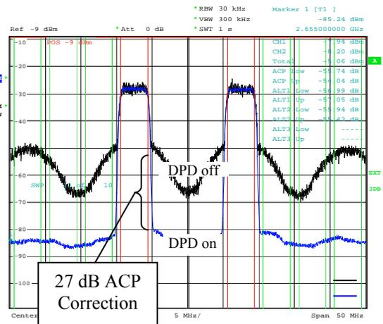
Figure 14: Graph showing Doherty amplifier performance with and without DPD applied for 10 dB PAR, 2.69 GHz W-CDMA signal at 80W average output power, 44.5% drain efficiency.
