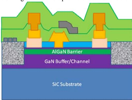
Figure 2: Schematic cross section of GaN HFET device.
