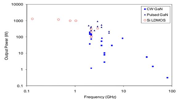
Figure 1: Output power versus frequency for GaN and Si LDMOS devices.
