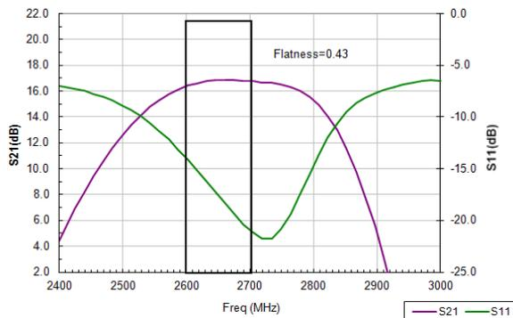
Figure 12: Graph showing measured S21 and S11 for Doherty power amplifier of Figure 11.
