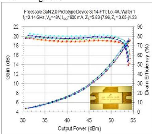
Figure 8: Saturation characteristics over power for a single 37.8 mm die in a NI-780-2 package under 2.14 GHz, 48V pulsed RF conditions in class A-B (600 mA  $I_{DQ}$ ) operation.
