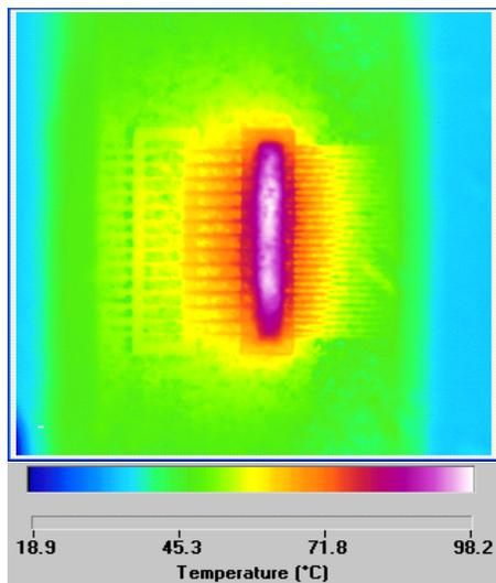
Figure 15: Thermal image of 200 W device of Figure 7(a) showing a thermal resistance of approximately 1 °C/Watt.
