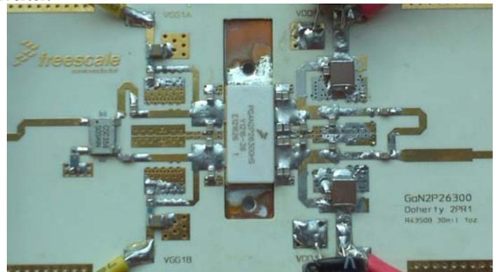
Figure 11: Realized 400 W GaN inverted Doherty PA using single dual path device. Effective circuit area is 2.4" X 3.4" (8 in<sup>2</sup>).
