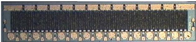
Figure 3: Die photo of a 37.8 mm GaN HFET die. Chip size is 4.7 x 1 mm<sup>2</sup>.
