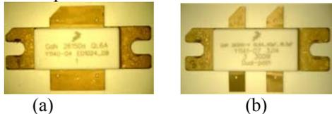
Figure 7: Photograph of (a) single and (b) dual path packaged transistors using NI-780 package footprints.
