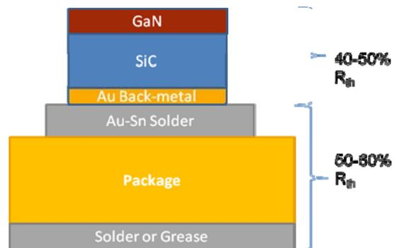
Figure 18: Schematic of materials stack for a packaged GaN HFET transistor.
