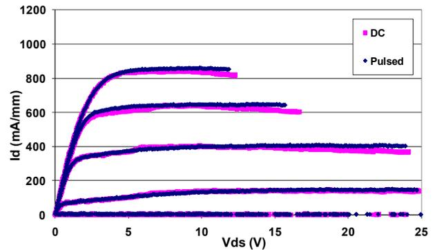
Figure 4: Comparison of DC and pulsed IV curves for 0.3 mm GaN HFET measured at a 10 W/mm power compliance at  $V_{DS}=0-20V$ ,  $V_{GS}=-5V$  to  $+1V$  in 1 V steps.
