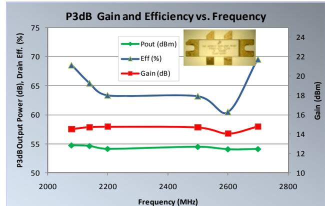
Figure 10: Over-frequency characteristics at  $P_{3dB}$  for a single 37.8 mm die in one path of an NI-780-4 package under 2.14 GHz, 48V pulsed RF conditions in (a) class A-B (600 mA  $I_{DQ}$ ) and (b) class C operation.
