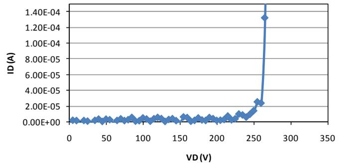
Figure 5: Small-device off-state breakdown characteristics for 0.15 mm GaN HFET device biased at  $V_{GS}=-5V$ .
