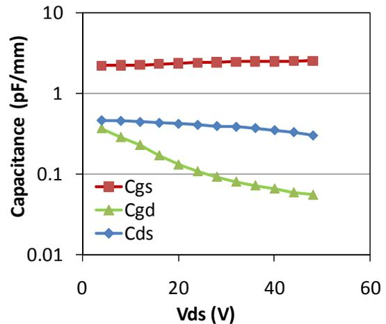
Figure 6: Small-signal capacitance versus drain bias characteristics of a 0.3 mm GaN HFET device biased at a quiescent current of 40 mA/mm.
